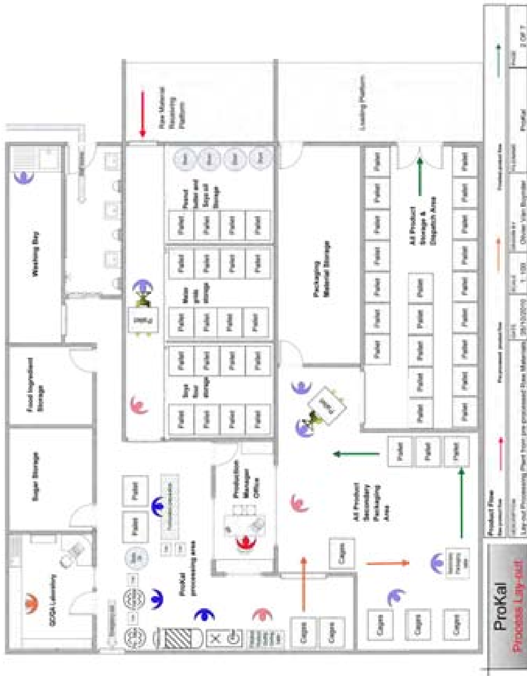
Figure 6: Layout of processing plant for manufacture of ProKal products from pre-processed raw materials
