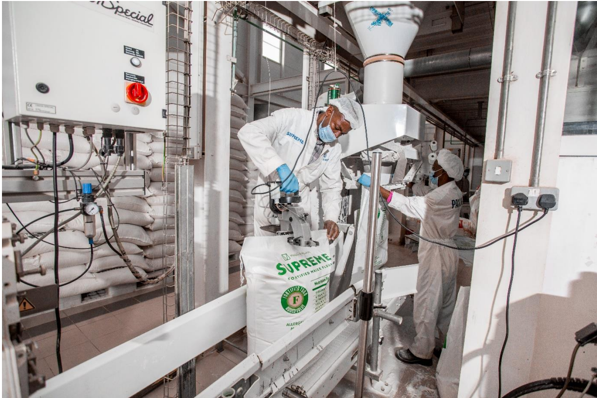
Photo credit: USAID Advancing Nutrition Uganda. Production personnel at Mandela Millers Limited sealing a 25 kg bag of fortified maize flour.
